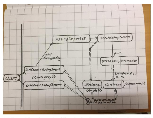
AssimpImporter is the most important class which transforms the assimp scene graph to the scene kit scene graph. It does the transformation by doing a depth first traversal of the assimp scene graph and for each assimp node visited, it generates a scene kit node.
