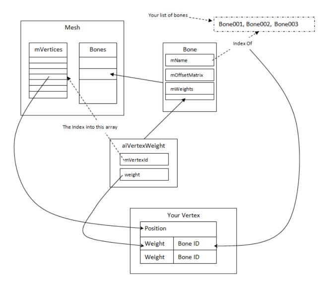
We parse the data structures above, so that we have a list of unique bone names, bone nodes and the bone inverse transforms. Once the unique bone nodes is known, the importer determines the root of the skeleton as that node which has the lowest depth from the parent!
