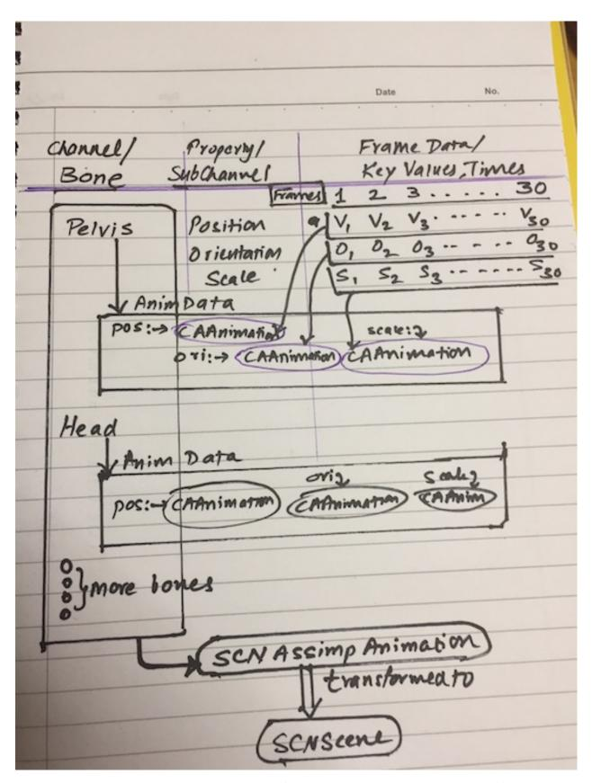
Each channel represents a bone and contains the keys for position, orientation and scale. The position, orientation
